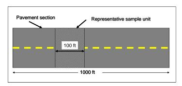
2. The area of AC sample units should be 2500±1500 square feet, and for PCC sample units, this should be 20±8 slabs. The total inspected area or slabs for a pavement section must be at least 10% of the total pavement section area or slabs. This is an exception to the procedure described in ASTM D6433.
